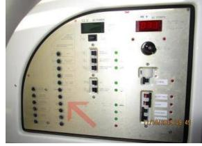
**Battery monitor:** Switched digital gauge to test battery condition.
